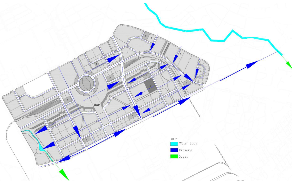
Figure 2-38: Proposed Drainage Scheme
